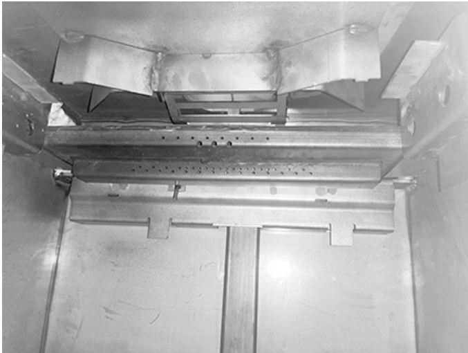
Figure 8: Remove rear baffle.
