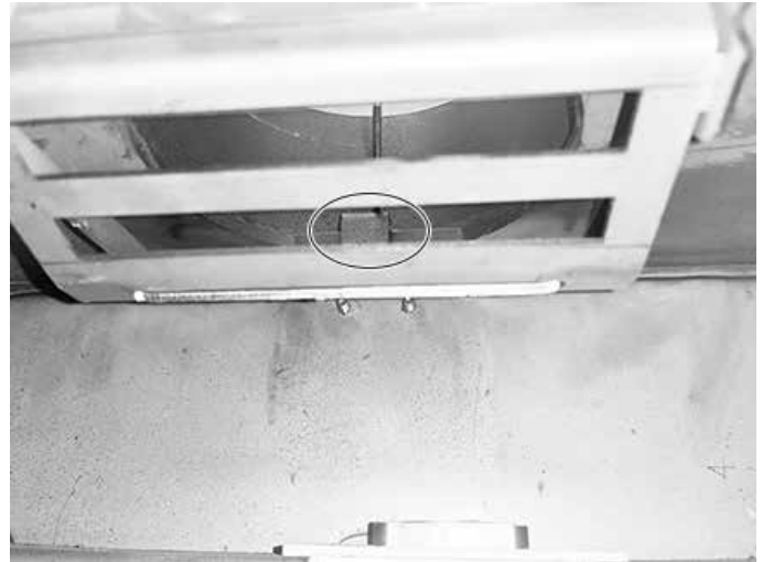
Figure 9: Remove Flue Gas Agitator
