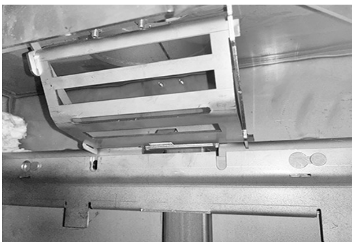
Figure 10: Lower agitator down.
