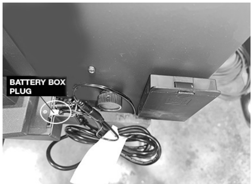
Figure 22: Plug in battery box.
